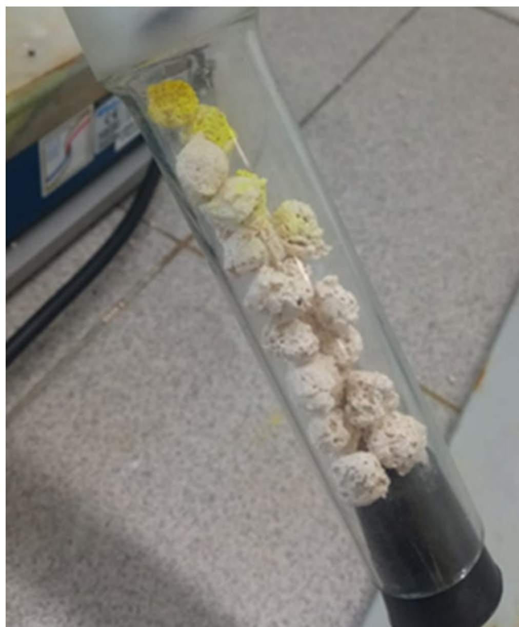
Fig.1.Change in color of the indicator sorbent during the experiment
