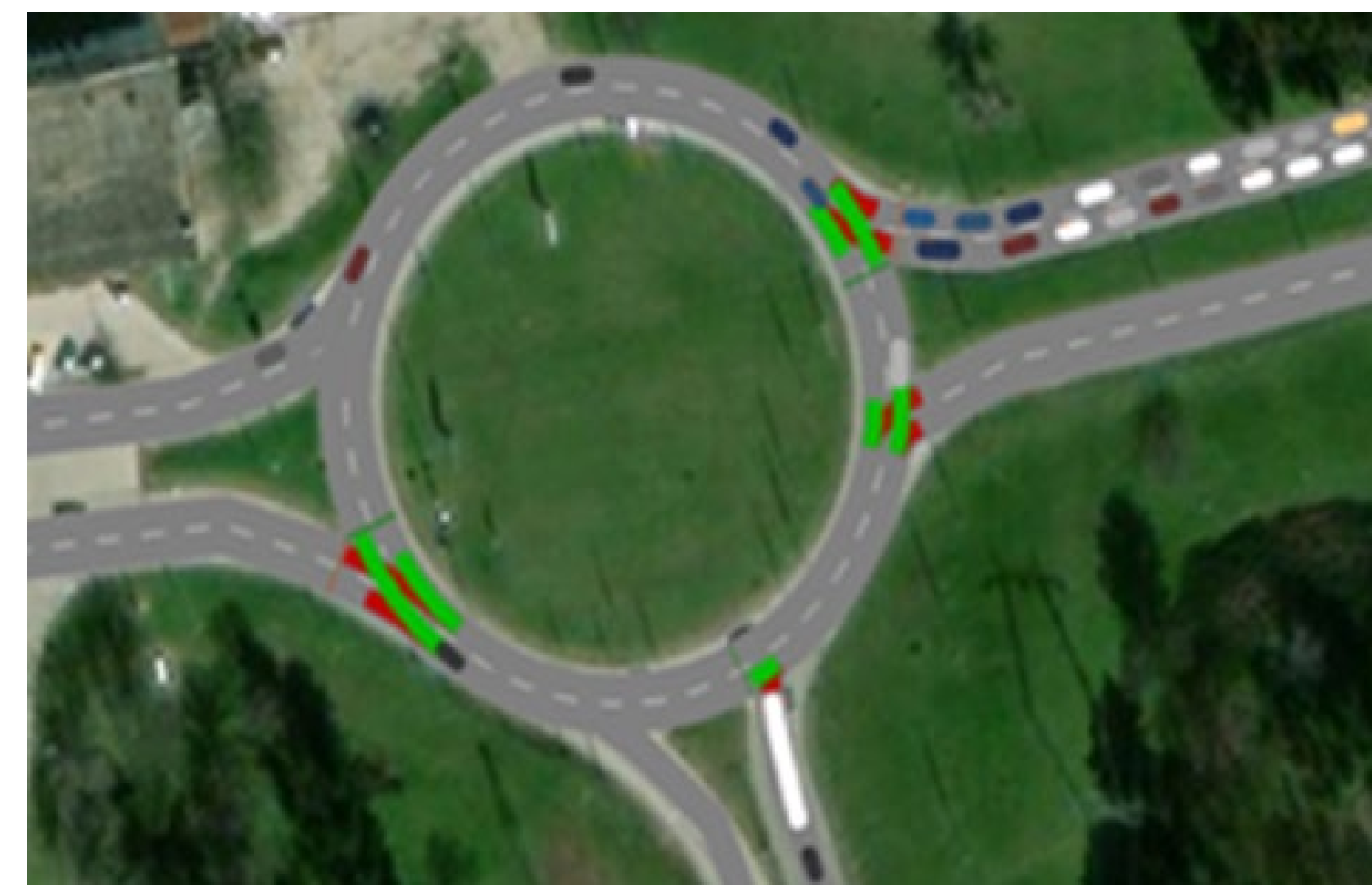
Fig. 2. Using a real-world map as a background layer for intersection scaling in PTV VISSIM.
