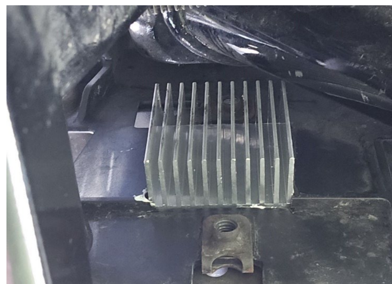
Fig. 2. Aluminum cooler with 11 fins, bonded to the Peltier element.
